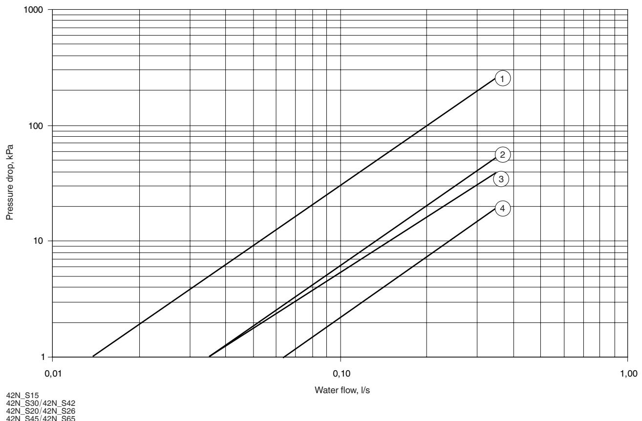
Heating conditions (entering water temperature = 50°C)
