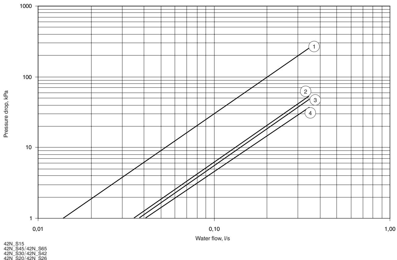
Heating conditions (entering water temperature = 70°C)
