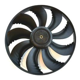
The 30RB/30RQ unit uses Carrier's sixth generation Flying bird™ fan technology, engineered for maximum efficiency, super low noise, and a wide operating range. The fans use Carrier patented rotating shroud technology and back-swept blades with a wave-serration trailing edge inspired by nature.
