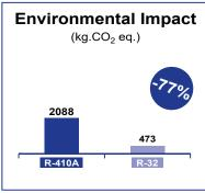
(1) Reduced refrigerant charge in Carrier heat pumps thanks to the use of R-32 and a new coil design.
